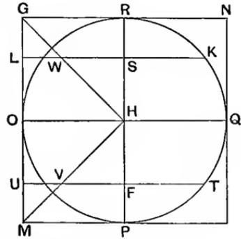
Through  $LK$ ,  $UT$  draw planes at right angles to  $PR$ , producing them on both sides of the plane of the circle; these planes produce as sections in the half cylinder  $PQR$  and in the prism  $GHM$  four parallelograms in which the heights are equal to the axis of the cylinder, and the other sides are equal to  $KS$ ,  $TF$ ,  $LW$ ,  $UV$  respectively.....
