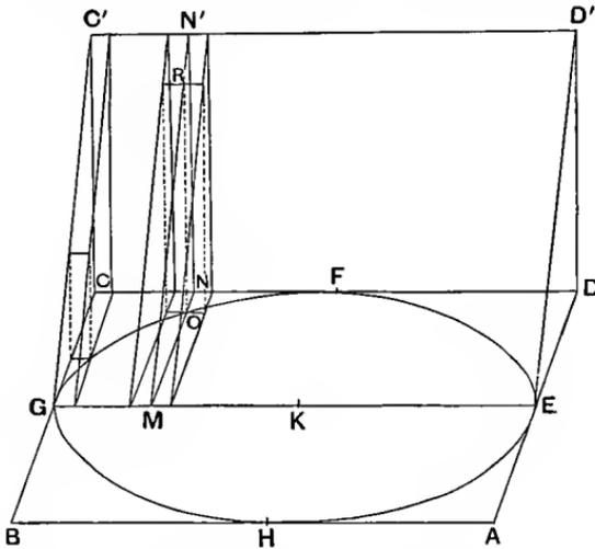
element-prism circumscribed to the portion of the cylinder, (2) two element-prisms adjacent to the ordinate  $OM$ , of which that on the left is circumscribed and that on the right (equal to the other) inscribed, (3) the corresponding element-prisms forming part of the prism cut off ( $CC'GEDD'$ ) which is  $\frac{1}{4}$  of the original prism.
