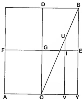
Let  $CD$  be the axis of the prism and cylinder, let  $EF$  bisect it at right angles, and through  $EF$  let a plane be drawn at right angles to  $CD$ ; this plane will cut the prism in a square and the cylinder in a circle.
