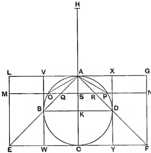
Draw straight lines from  $A$  to the four corners of the section in which the plane through  $BD$  perpendicular to  $AK$  cuts the cube. These straight lines, if produced, will meet the plane of the face of the cube opposite to  $A$  in four points forming the four corners of a square in that plane with sides equal to  $EF$  or double of the side of the cube, and we thus have a pyramid with  $A$  for vertex and the latter square for base.
