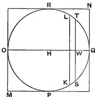
Let  $KL$  be the intersection of the plane through  $EF$  perpendicular to the axis of the cylinder and the plane cutting off the portion of the cylinder;  $KL$  is bisected by  $OHQ$  [and passes through the middle point of  $HQ$ ].
