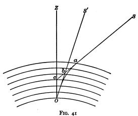
Fig. 41, S is the true position of a star and S' its apparent position. The light from S is bent into a curve aO, and the star is seen in the direction of the tangent ObS'. The angle which must be subtracted from the altitude of S' to obtain the altitude of S is called the refraction correction. This angle is really the angle SOS', but on account of the great distance of celestial objects
