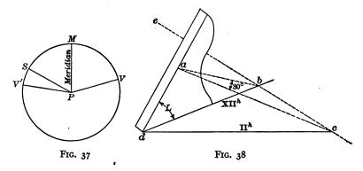
3. Make a design for a horizontal sun dial for a place whose latitude is 42° 21′ N. The gnomon ad (Fig. 38), or line which casts the shadow on the horizontal plane, must be parallel to the earth's rotation axis; the angle which the gnomon makes
